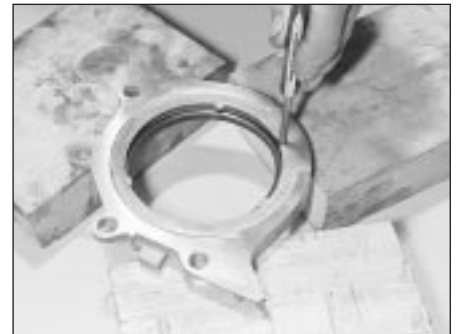
20.13 . . . and ensure that carrier is properly supported when driving out used oil seal - note notches provided in carrier for drift
