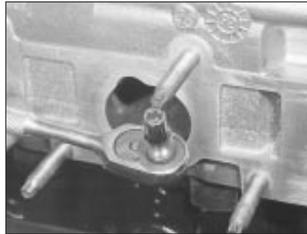
7.9B . . . studs can be unscrewed also, if required, to provide additional working space
