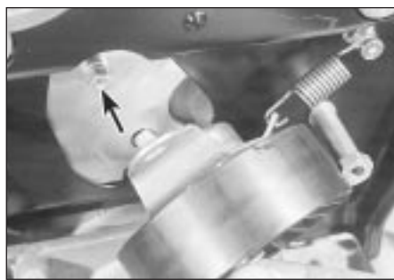
10.19B Hook spring onto tensioner and refit as shown - engage tensioner backplate on locating peg (arrowed) . . .
