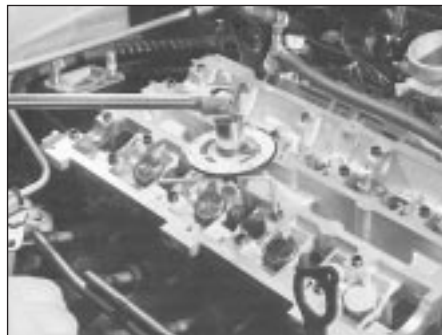
14.32B . . . and to third stage using angle gauge
