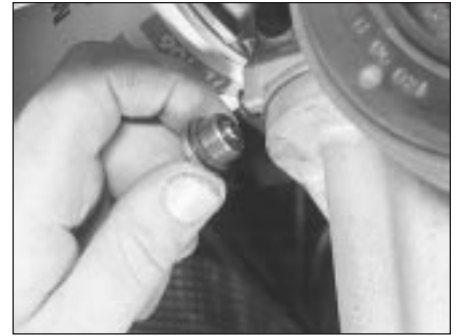
16.9A Unscrew threaded plug - seen through right-hand wheel arch . . .
