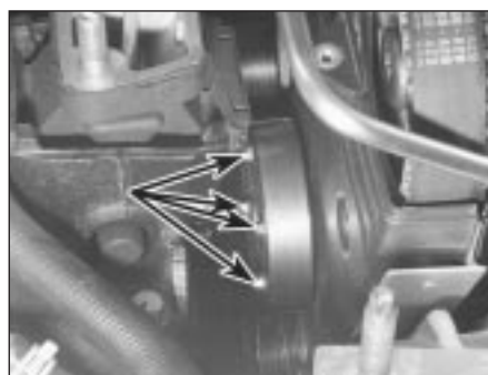
9.7 Slacken water pump pulley bolts and remove pulley
