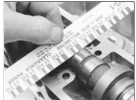
13.13B Compare the width of the crushed Plastigage to the scale on the envelope to determine the running clearance
