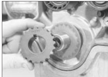
11.8 Note "FRONT" marking on outside face of crankshaft toothed pulley - note which way round thrustwasher behind is fitted
