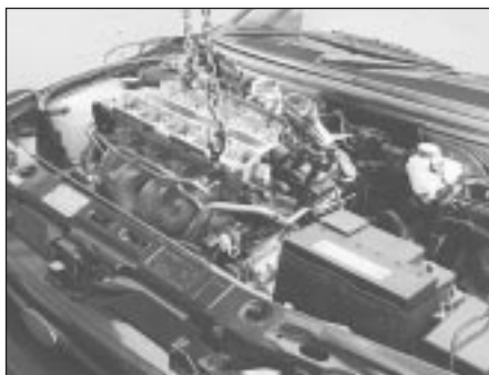
14.22 Using an engine hoist to lift off the cylinder head complete with manifolds
