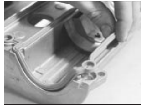
5.8 Ensure gasket is located correctly in cover groove
