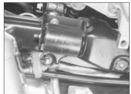
22.16 Where vehicle is fitted with automatic transmission, additional damper may be fastened to underside of engine/transmission rear mounting, as shown
