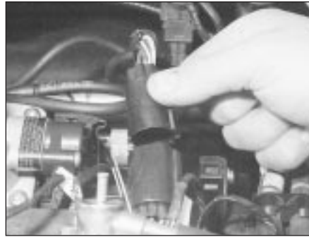
14.8A Release wire clip to unplug engine wiring loom connector from inlet manifold
