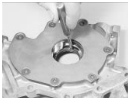
20.2 Driving out crankshaft right-hand oil seal
