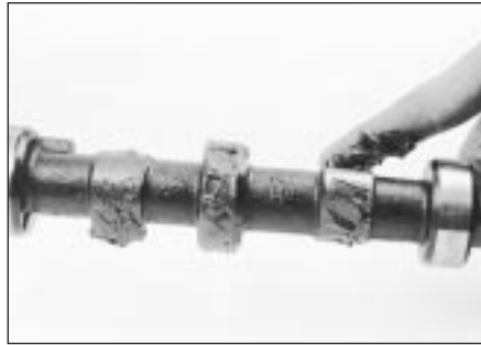
13.18A Apply engine assembly lubricant or molybdenum disulphide-based grease to the cam lobes and journals before refitting a camshaft
