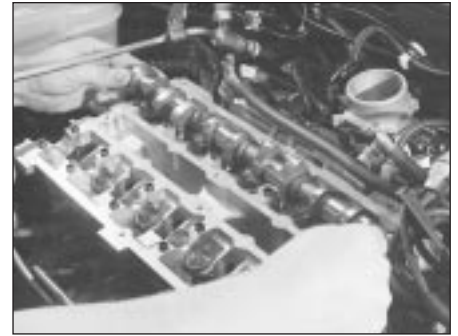
13.18B Use camshaft position sensor lobe to identify inlet camshaft on refitting - locate camshafts as described in text
