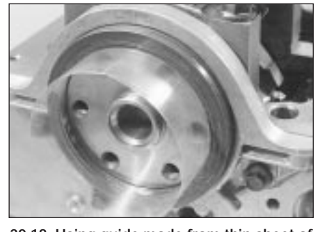
20.18 Using guide made from thin sheet of plastic to slide oil seal lips over crankshaft shoulder
