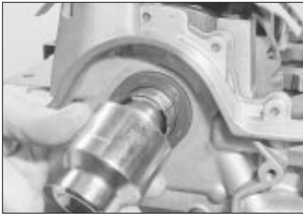
20.5 Socket of correct size can be used to replace Ford service tool, drawing new seal into place as described
