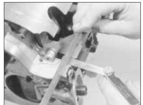
16.13 Check the oil pump is positioned correctly
