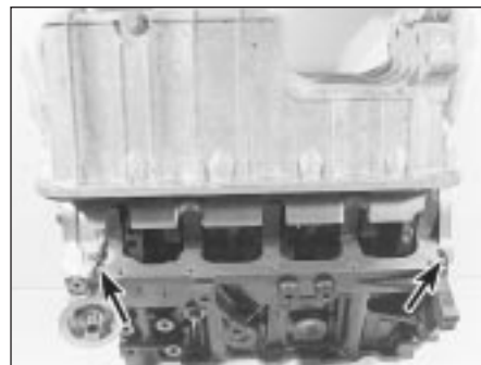
15.19A Apply sealant (arrowed) as directed when refitting sump
