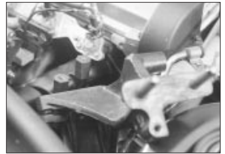
6.15 Alternator mounting bracket must be unbolted from rear of cylinder block to permit access to inlet manifold nut
