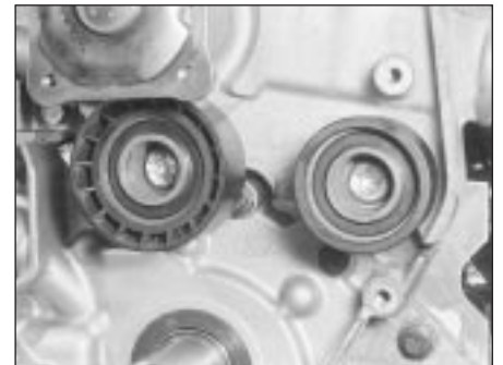
11.13 Tighten timing belt guide pulley bolts to specified torque settings on refitting
