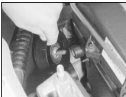
14.17 Unbolt auxiliary drivebelt idler pulley
