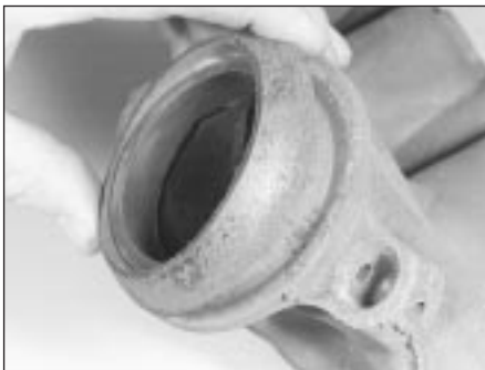
7.13B Renew exhaust system downpipe-to-manifold gasket to prevent leaks
