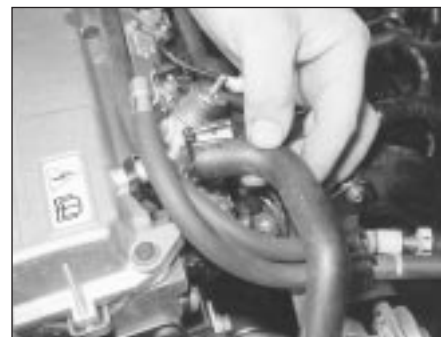
5.4 Disconnecting crankcase breather hose from cylinder head cover union
