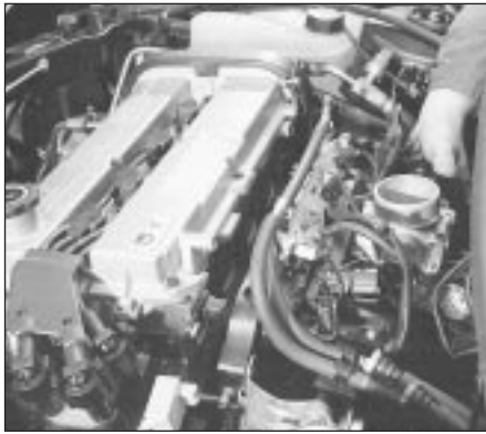
6.16 Withdrawing inlet manifold - take care not to damage delicate components
