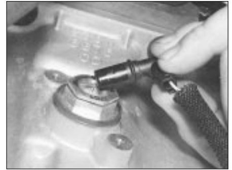
18.4 . . . disconnecting wiring from sensor
