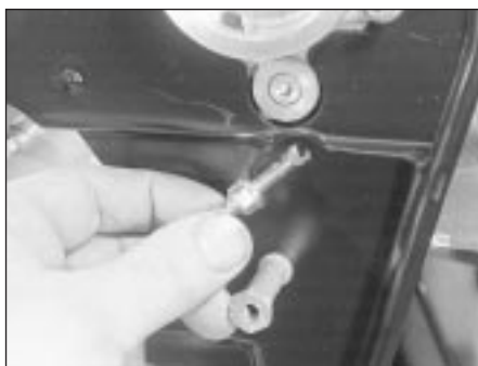
10.19A Fitting tensioner spring retaining pin
