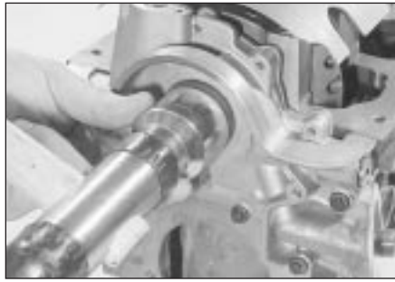
20.6 If seal is tapped into place as shown, exercise great care to prevent seal from being damaged or distorted
