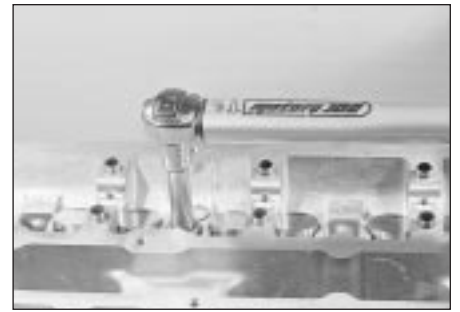
14.32A Tightening cylinder head bolts (to first and second stages) using torque wrench . . .
