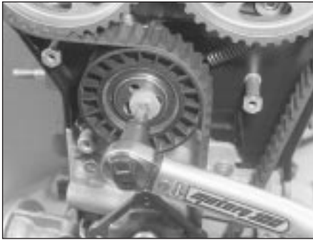
10.26 When setting is correct, tighten tensioner bolt to specified torque wrench setting
