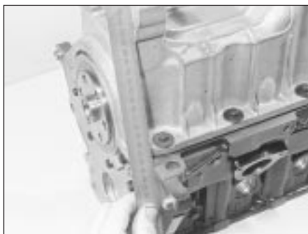
15.19B Checking alignment of sump with cylinder block/crankcase
