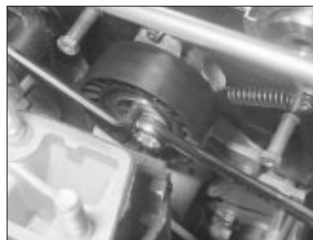
10.20 . . . then use Allen key to position tensioner so that timing belt can be refitted
