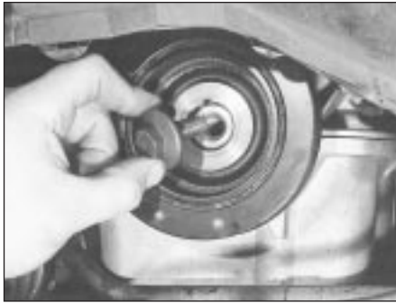
8.4A Unscrew pulley bolt to release crankshaft pulley
