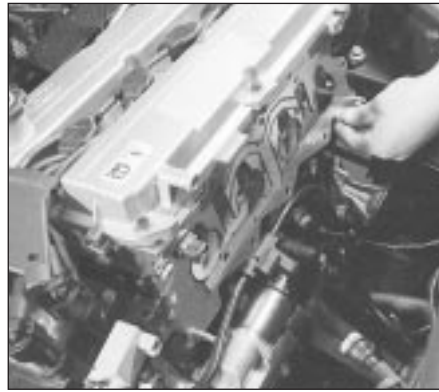
6.17A Always renew inlet manifold gasket - do not rely on sealants
