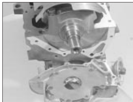
16.12 Use new gasket when refitting oil pump
